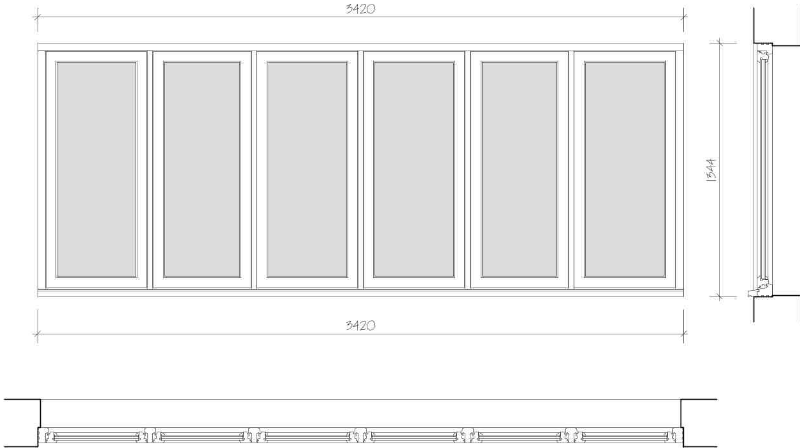
TYPICAL WINDOW DETAIL 1:20 (PAINTED SOFT WOOD)
