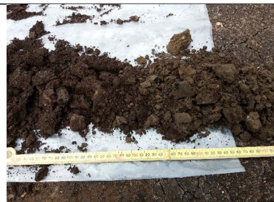
Photograph 2: Showing the difference between the clean cover and the underlying topsoil strata at HA2.
