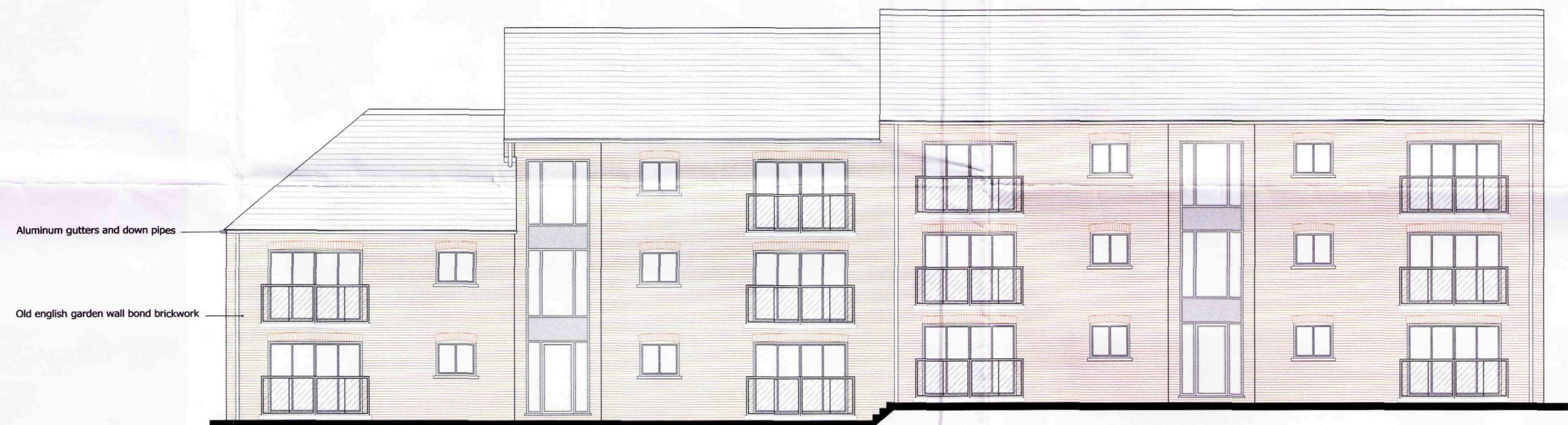
REAR ELEVATION - Block A
