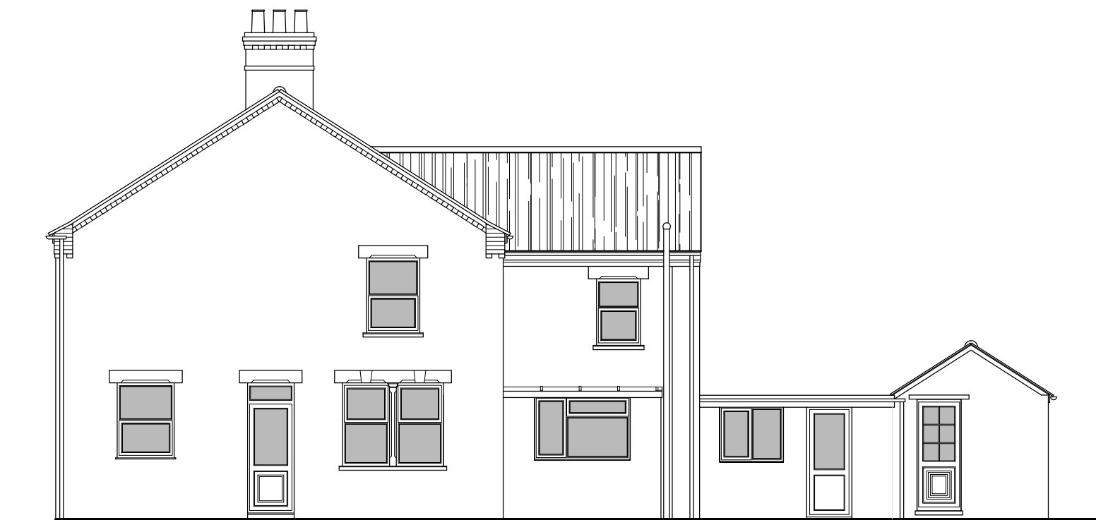
SOUTH - WEST ELEVATION
