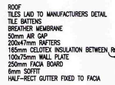
PITCHED ROOF EAVES DETAIL WITH SLOPING INSULATION
