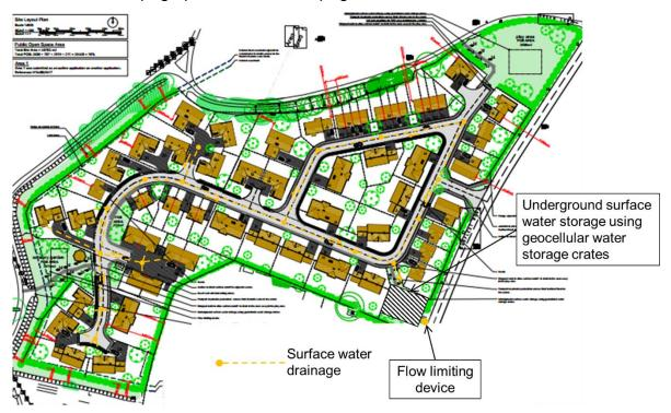
The surface water will flow southwards from the flow limiting device and discharge into the piped IDB drain at the junction of Milestone Lane and Surfleet Road.
