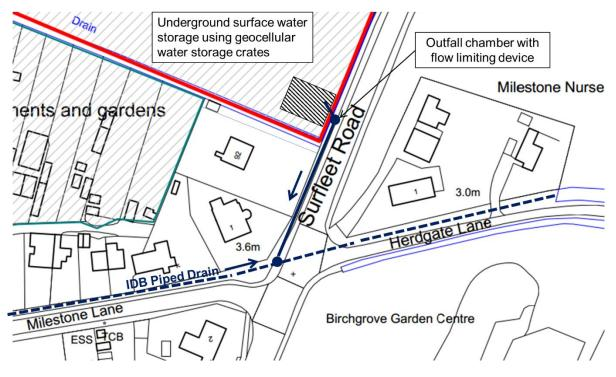
Total area of site = 4.07haThe impermeable areas of roads.......  $680 \times 7.5 = 5,100 \text{ sq m}$ Houses on plots 16 - 28 ......1,716 sq mTotal impermeable area ......6,816 sq m
