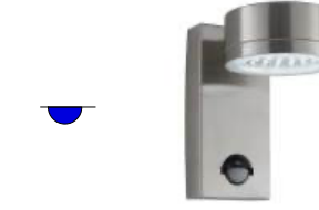
Indicates 9550SS LED wall/fence mounted downlighter Class 1 150mm high, 140mm protrusion built in motion sensor. Stainless steel. Runs with 36no 0.06w leds. These lights are 'Bat friendly'.
