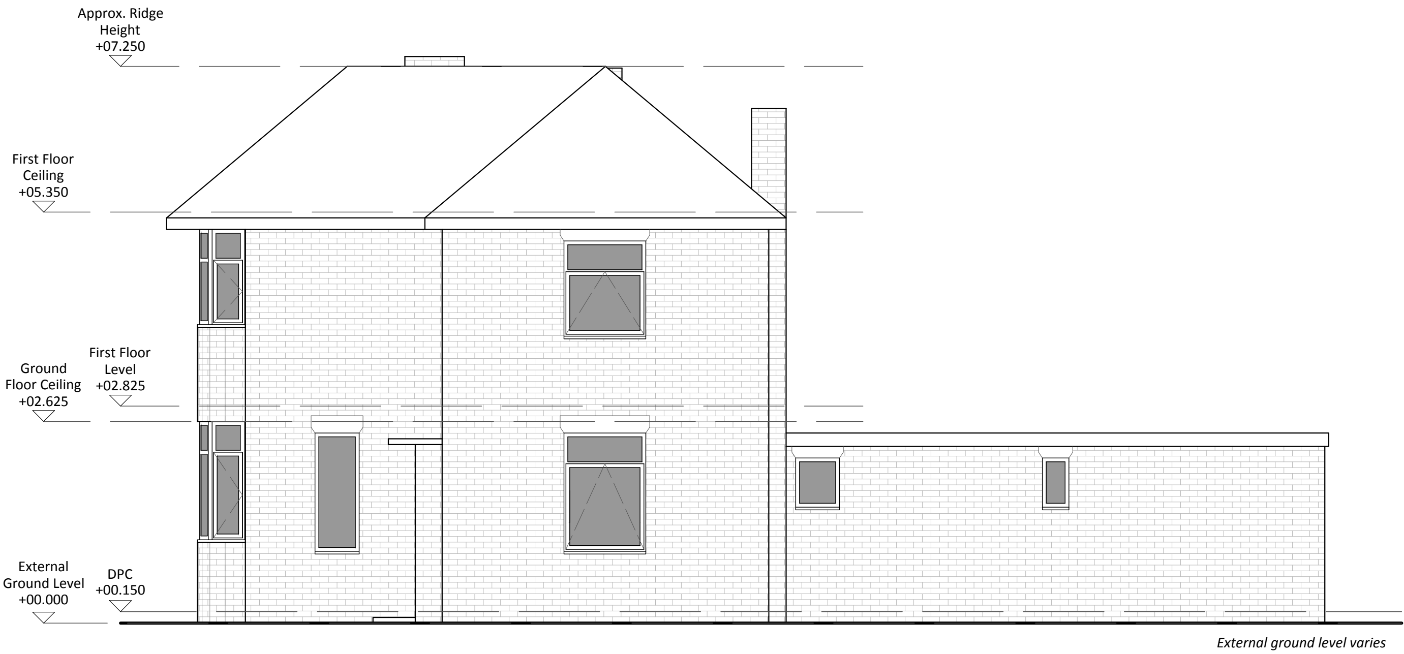
Existing Side (North-East) Elevation 1:50
