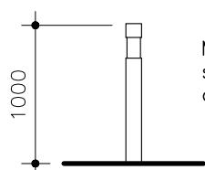
Marshalls Ref: RS150 stainless steel static anti-ram bollard with factory applied hazard banding
