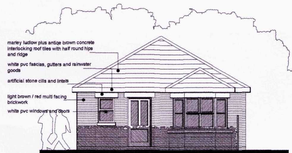
FRONT ELEVATION - West
