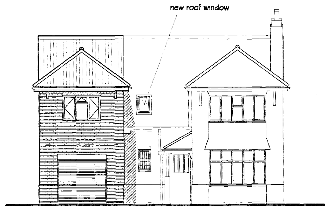
Proposed Front Elevation Scale 1/100
