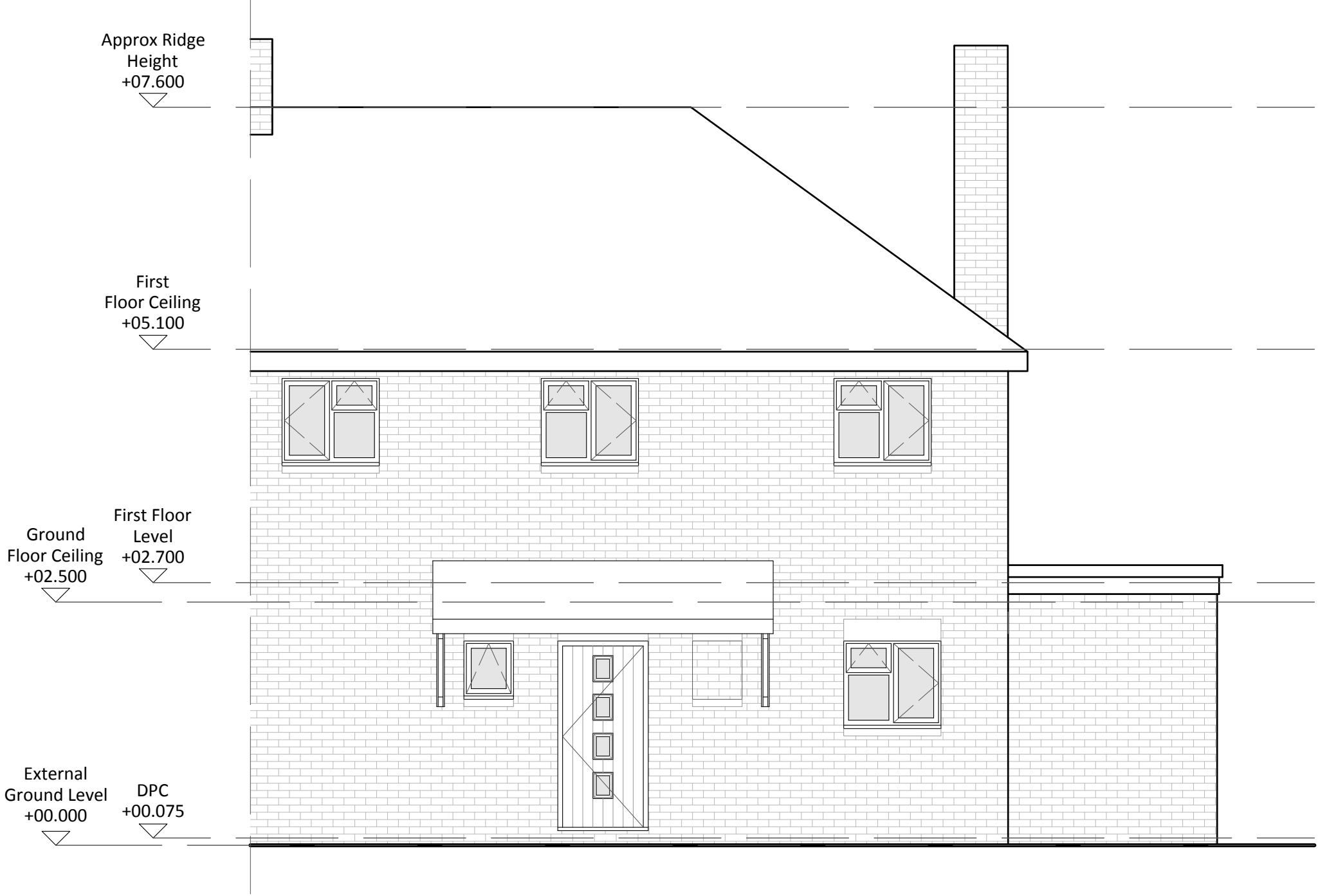
Proposed Front (West) Elevation 1:50
