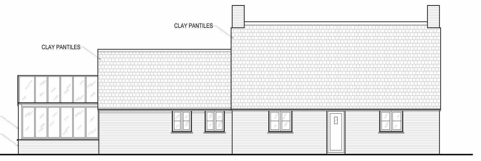
Rear Elevation (East) Existing - 1 to 100
