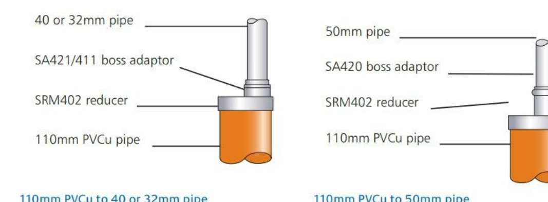
8. 32, 40 & 50mm connections to 110mm dia pipe.
