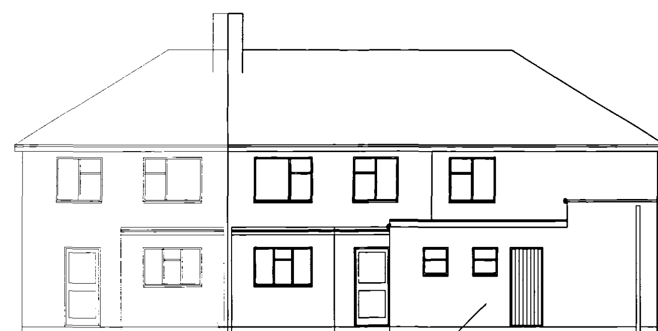
Rear Section to be Demolished
