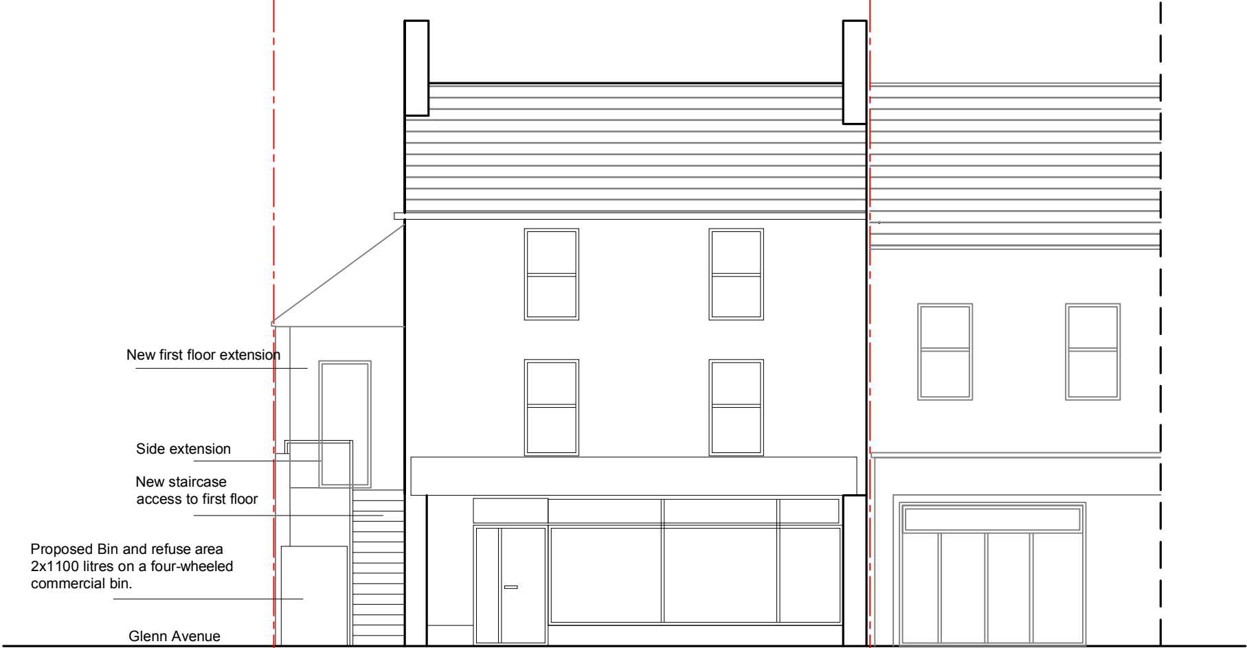
FRONT ELEVATION PROPOSED SCALE 1:100
