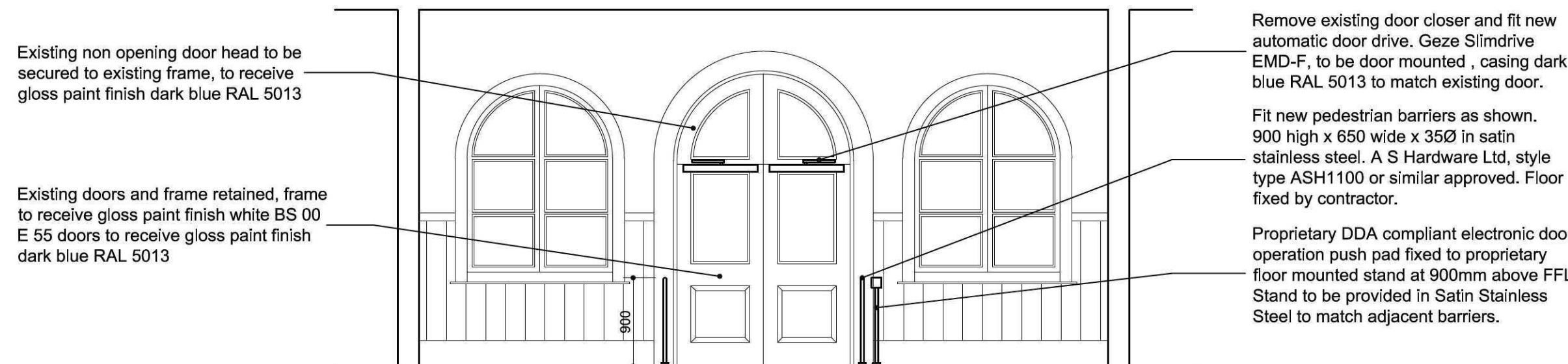
Proposed Auto Door Internal Elevation (Platform Door) (Scale 1:50)
