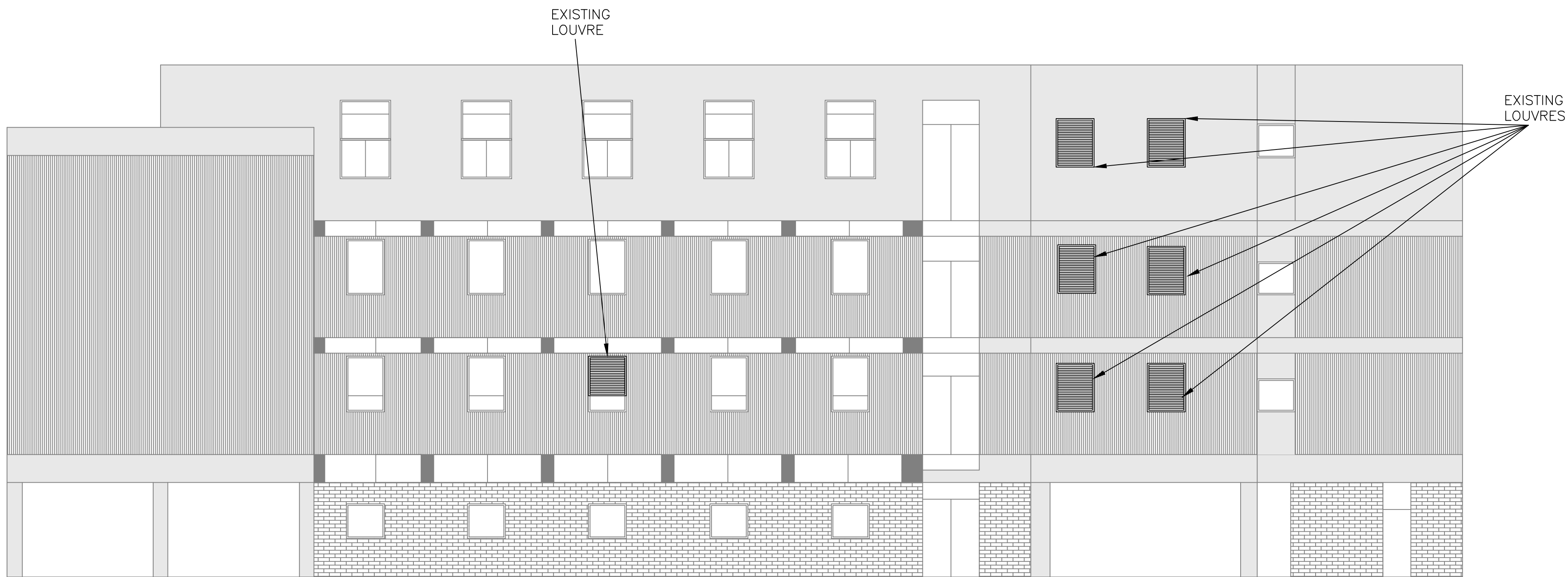
PROPOSED WEST ELEVATION (1:100)
