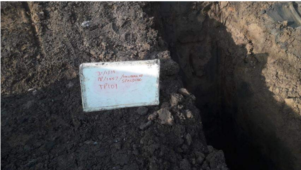
TP100 after collapse, exposed black organic/peaty laminations within the natural silt.
