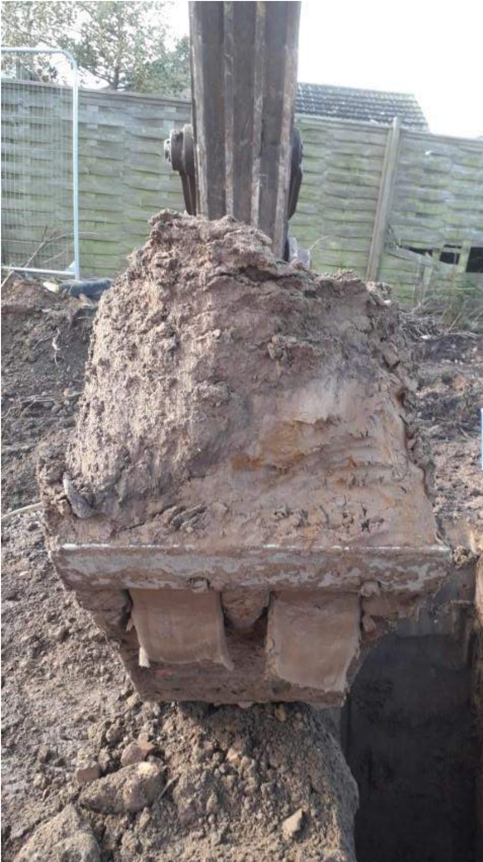
TP107, typical laminated estuarine sand deposits from near base.
