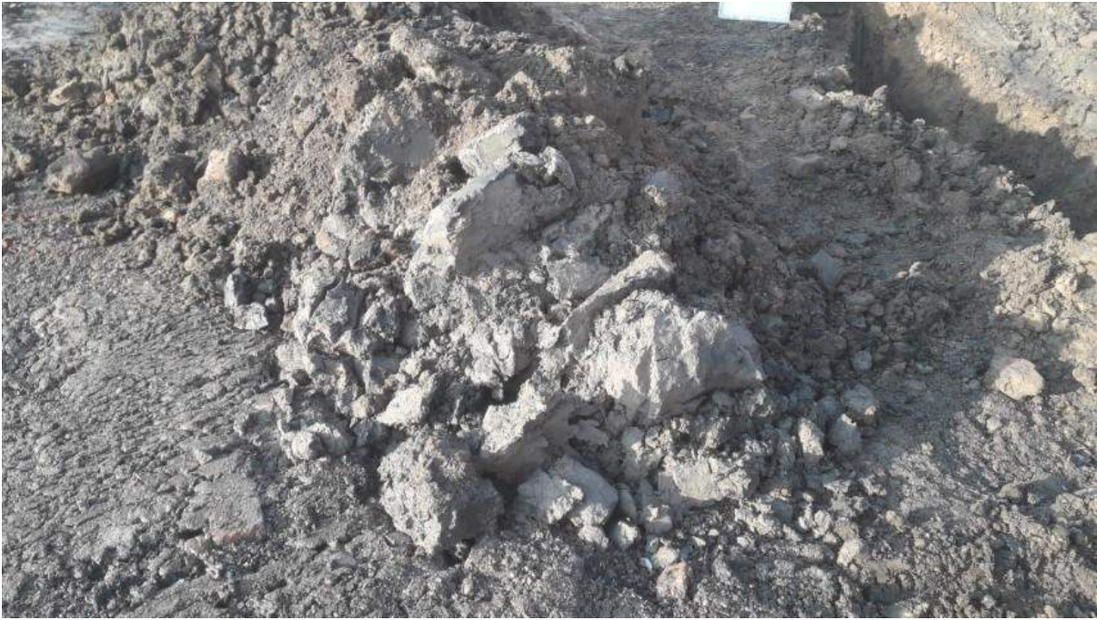
Typical natural estuarine deposits, excavated from trial pit TP101.
