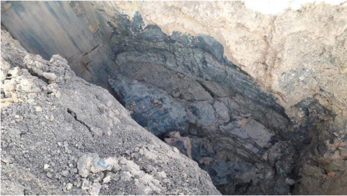
TP100 after collapse, exposed black organic/peaty laminations within the natural silt.
