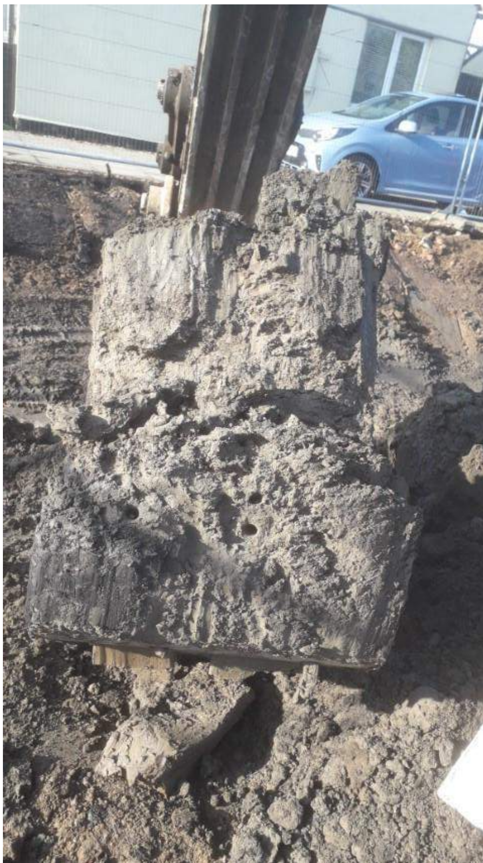
TP103, showing estuarine deposits. Holes are for PID probe.
