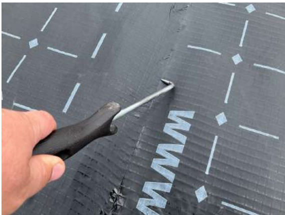
Plot 2. Pick testing along hand welded lap joints.
