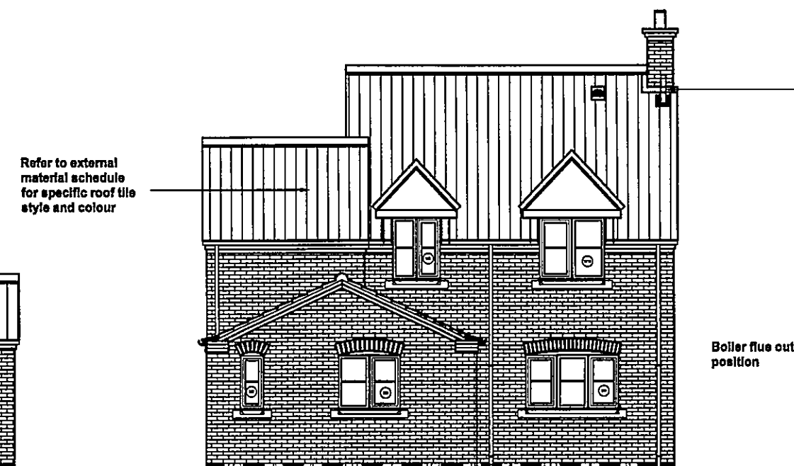
Rear Elevation - Plot-2 Scale 1:100
