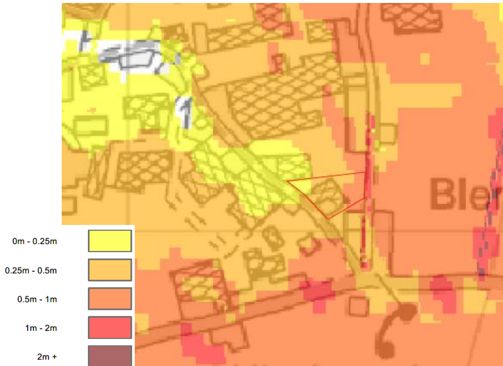
Fig.12: Residual Peak Flood Depth; Year 2115 1% Fluvial/0.5% Tidal (SEL SFRA Appendix B)
