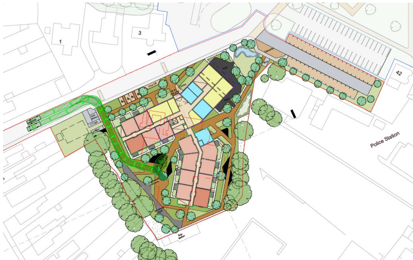
Image shows fire tender tracking within the garden area.
