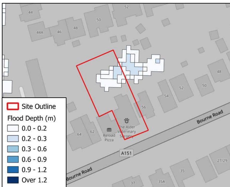
Figure 13 - Depth of surface water flooding, CC medium risk event (data from EA)
