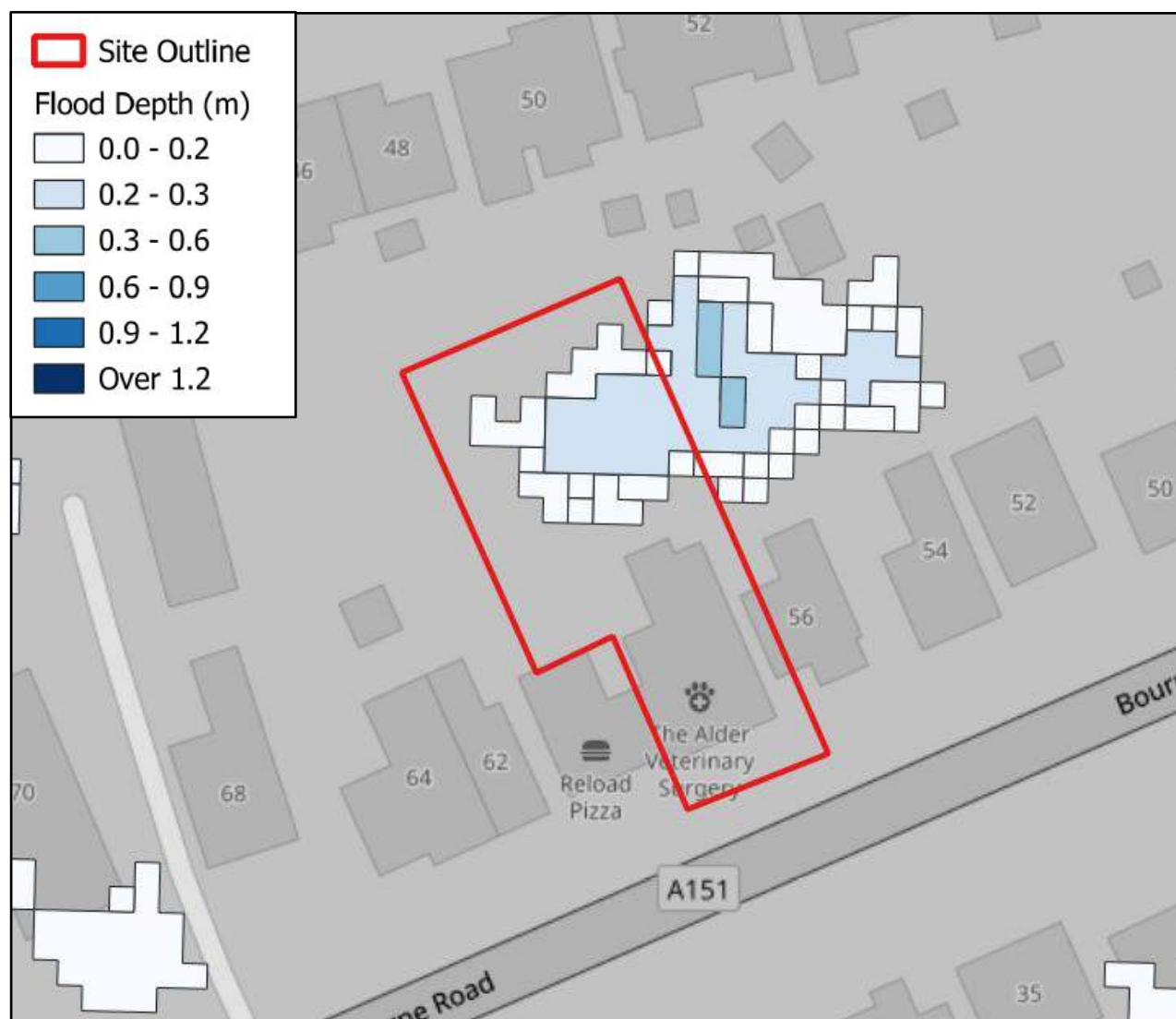
Figure 10 - Depth of surface water flooding, present day low risk event (data from EA)
