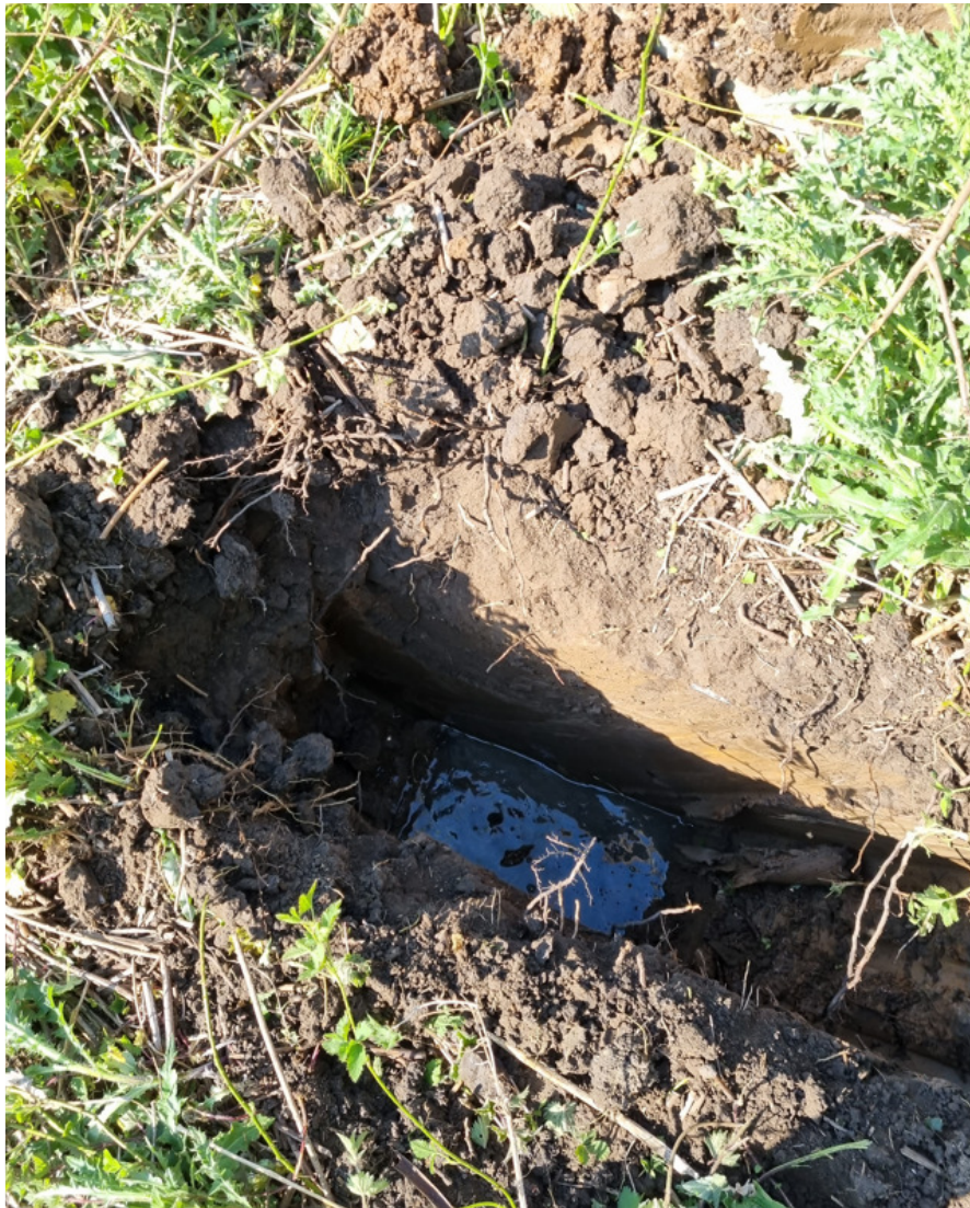
Figure 5 – Standing Water after 10 minutes – 900mm below ground level
