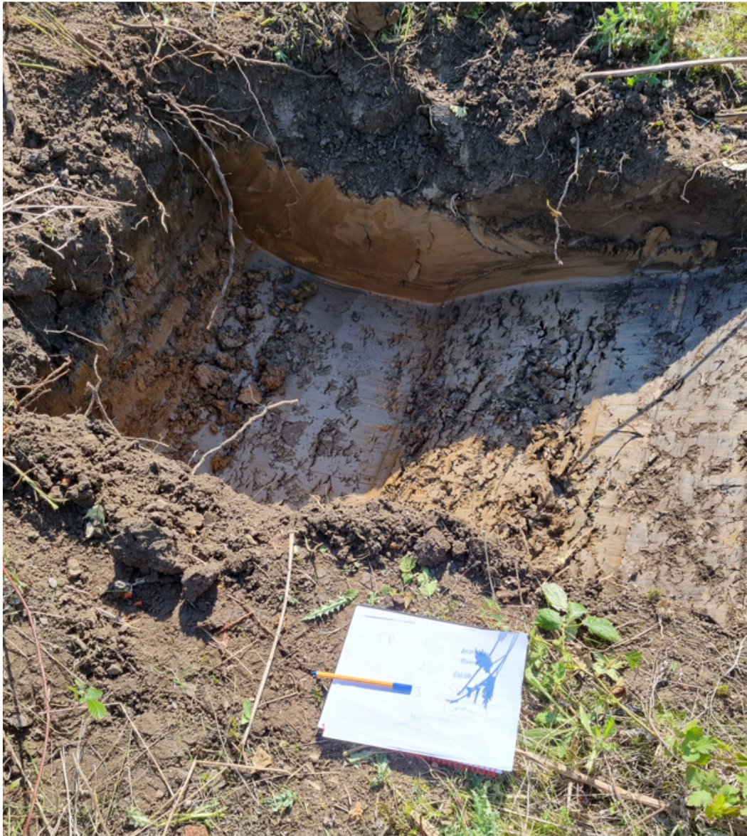
Figure 3 – First Recorded Trial Pit – Primarily Clay, 600mm Deep
