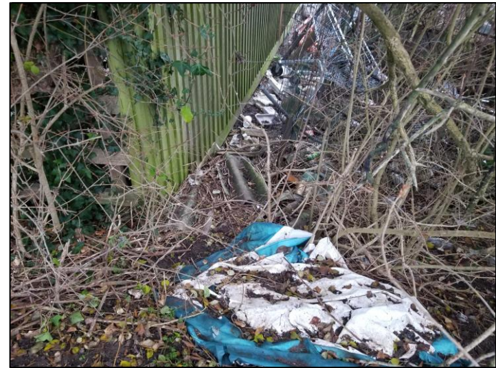
Photo 6 - Asbestos Sheetting Found in North-Western Corner.
