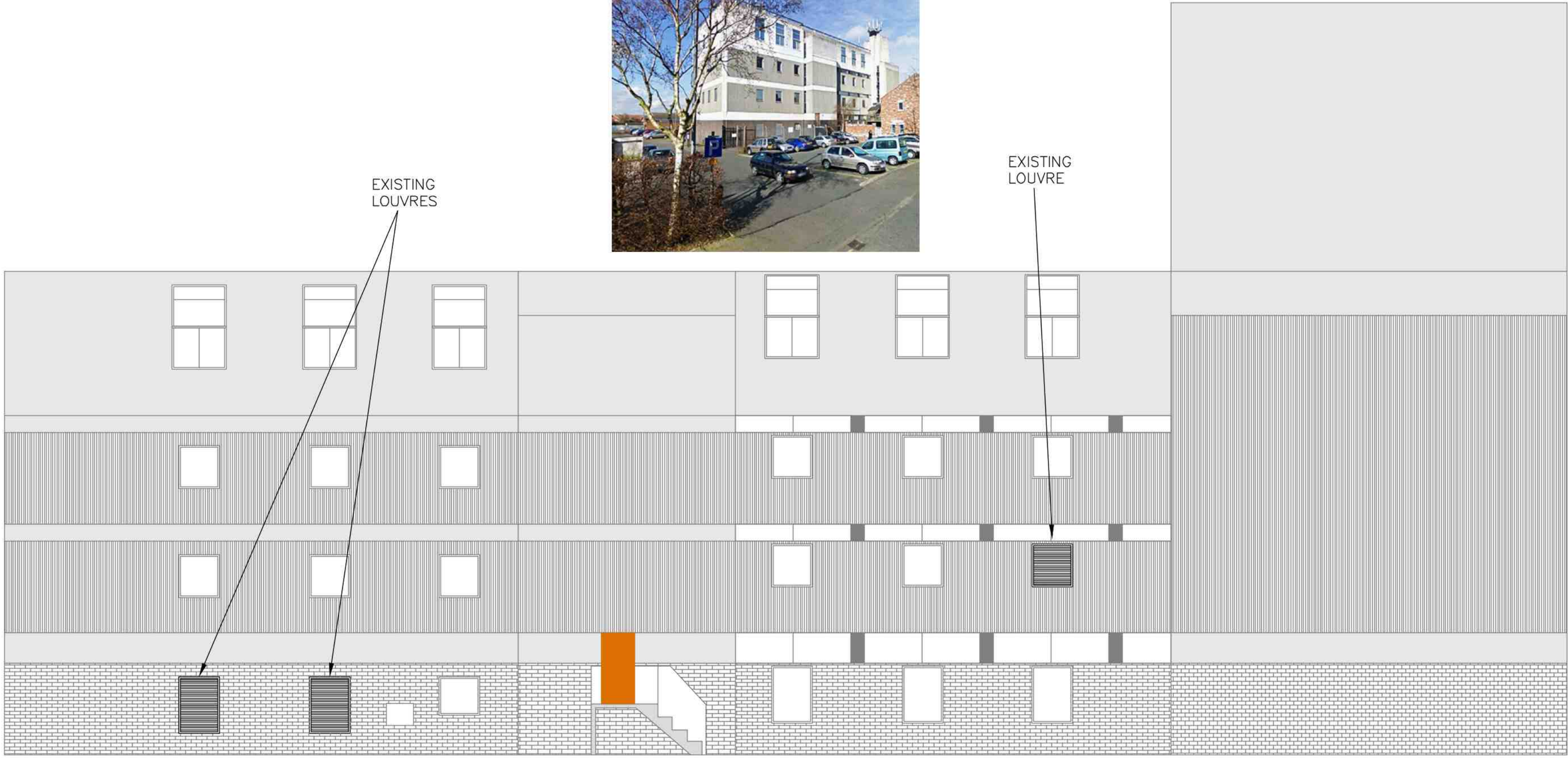
EXISTING EAST ELEVATION (1:100)
