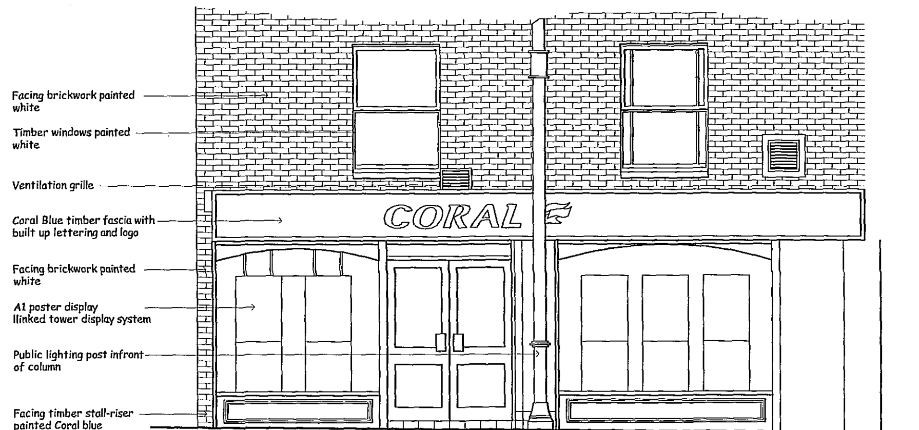
FRONT ELEVATION AS EXISTING
