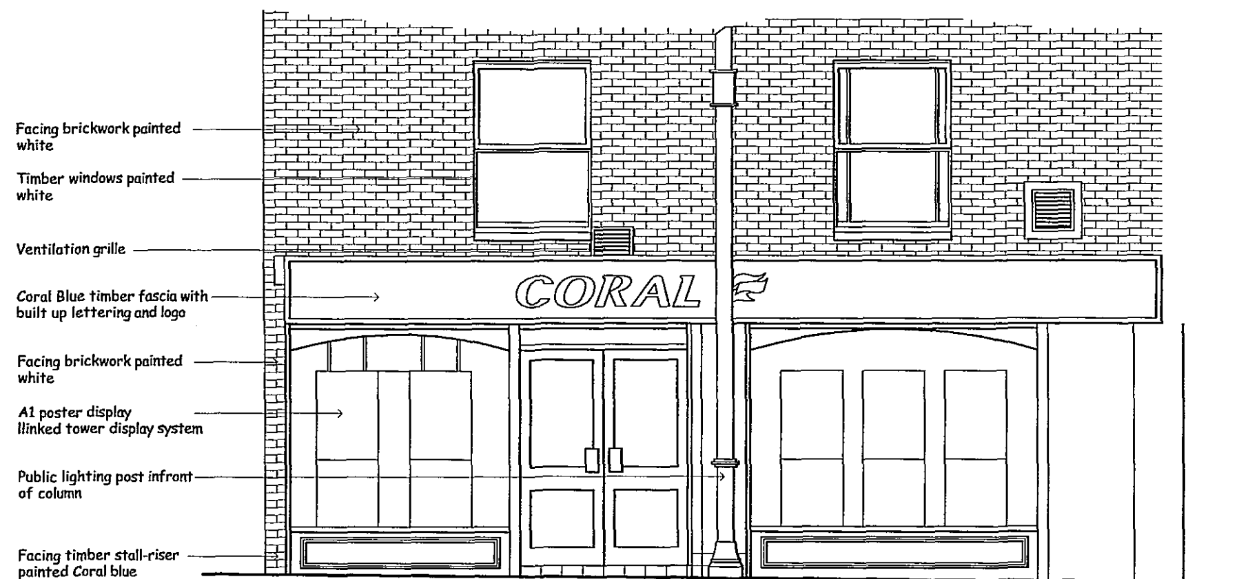
FRONT ELEVATION AS EXISTING
