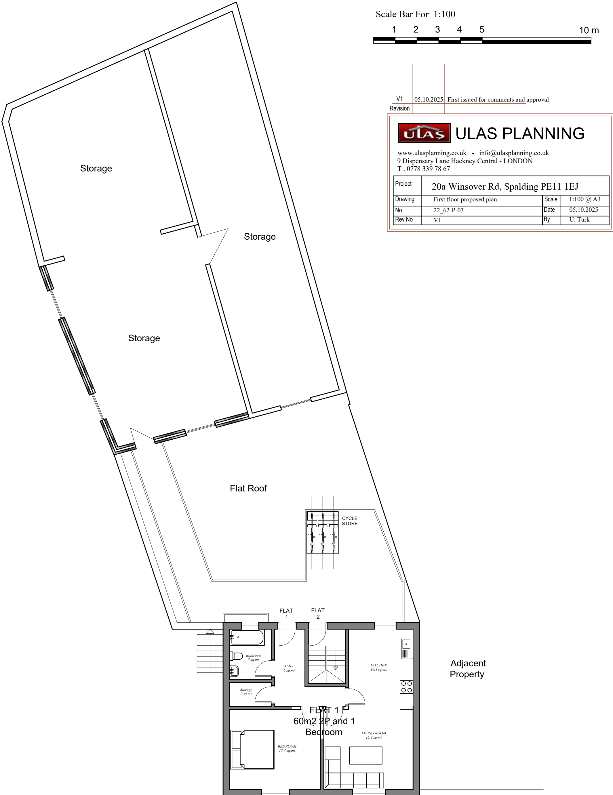
FIRST FLOOR PROPOSED SCALE 1:100
