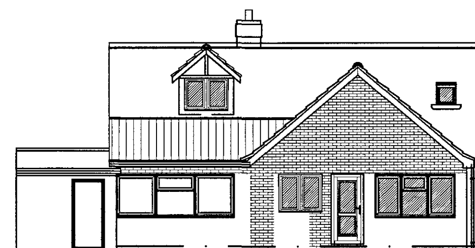
Proposed Rear Elevation Scale 1:100
