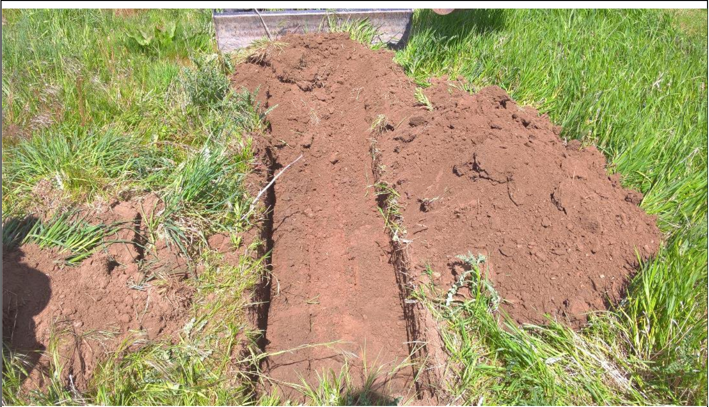
Photograph No.3: TP201 showing made ground topsoil with no anthropogenic inclusions.
