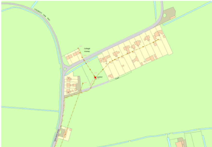
Figure 11 - Foul Connection into Newlands Road
