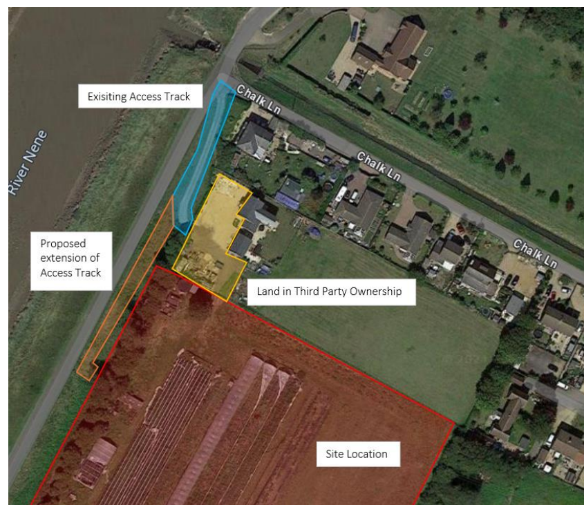
Figure 2: Existing and Proposed Access Arrangement
