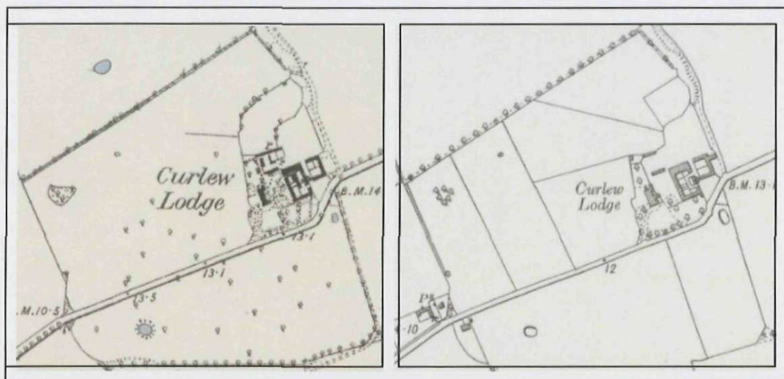
(Above) Fig.1b Extract from the six inch Ordnance Survey Maps of 1887 (left) and 1929 (right) showing changes in buildings associated with the main (central) ranges. The addition of division A (Fig. 4), currently used as a chicken shed is apparent on the southeast corner of the range by 1929.
