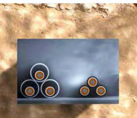
↑ Powercrete is used in the open ditch
