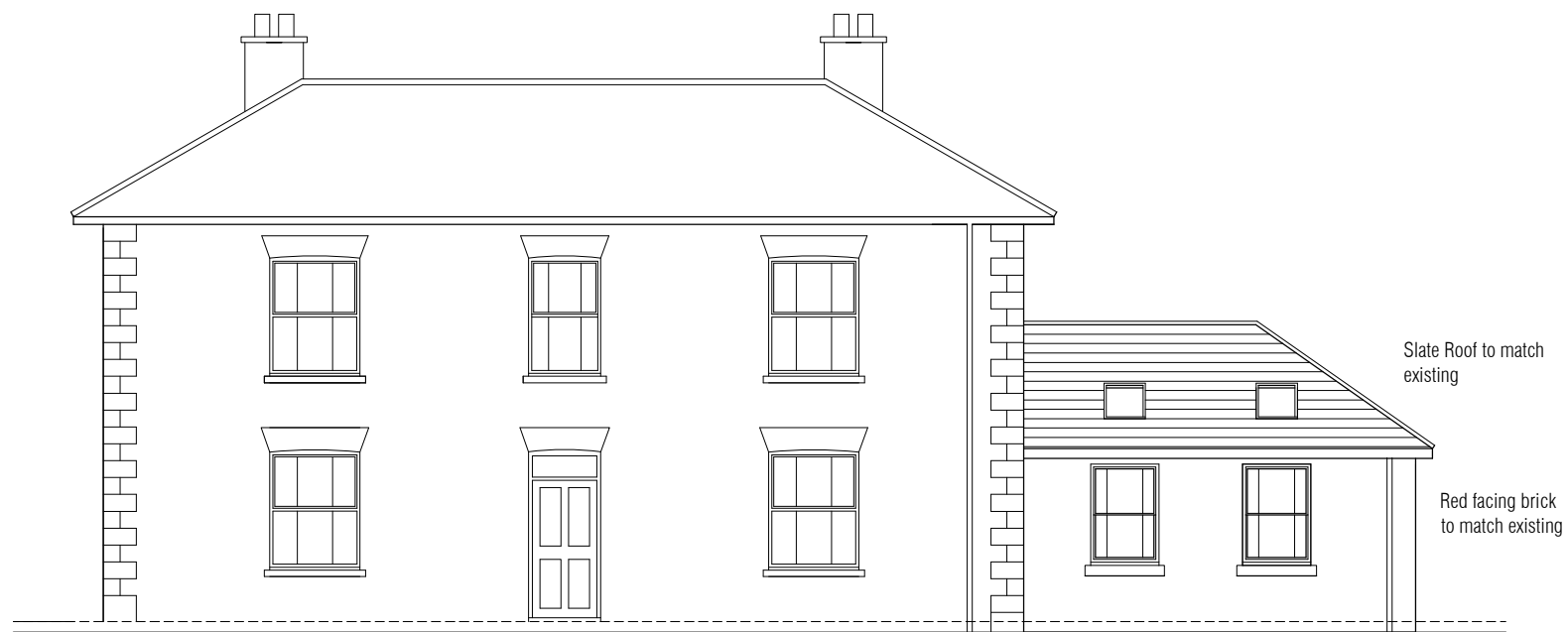
front elevation (west )
