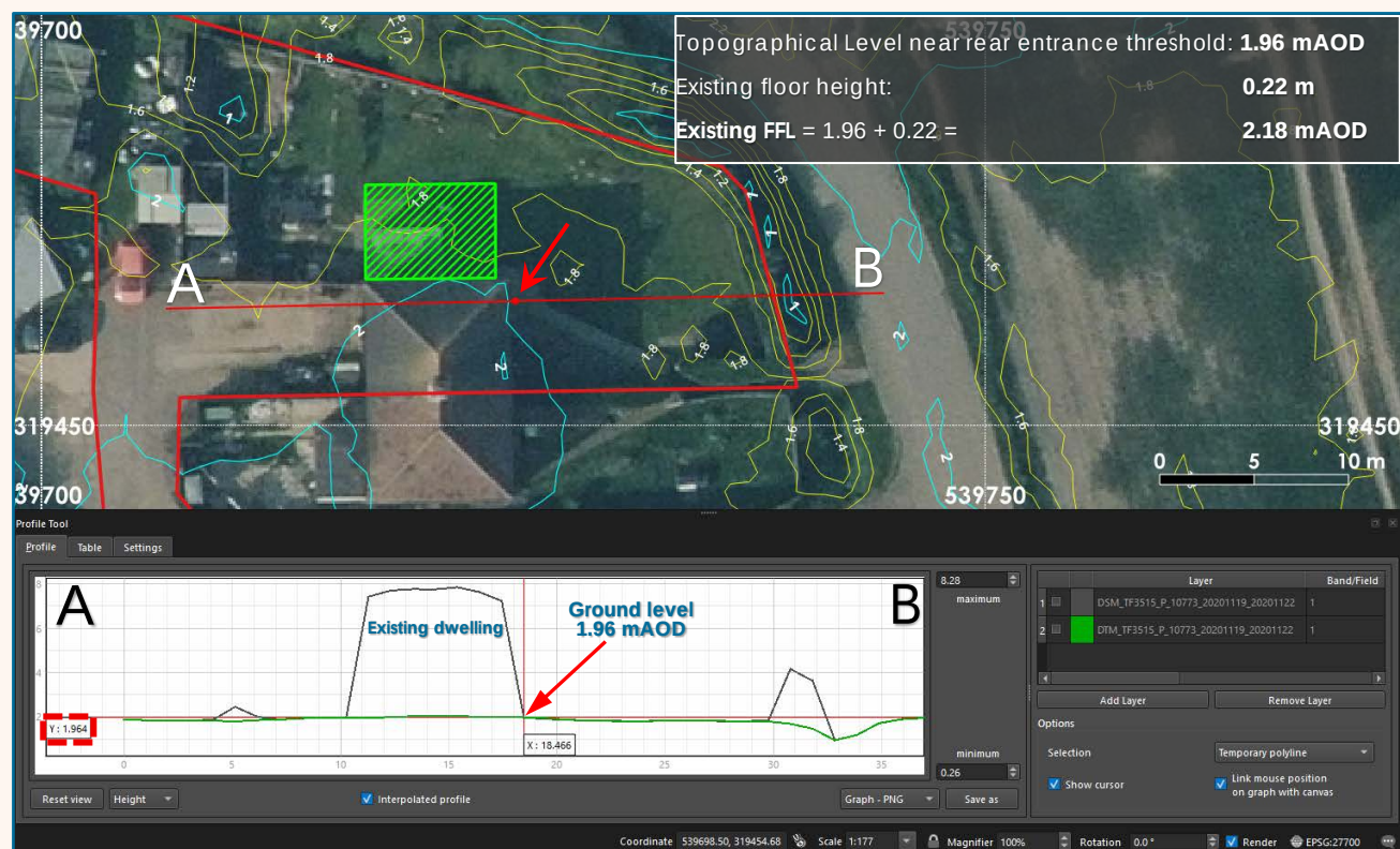
Figure 16: Cross-sectional analysis using Lidar to validate Floor Levels information
