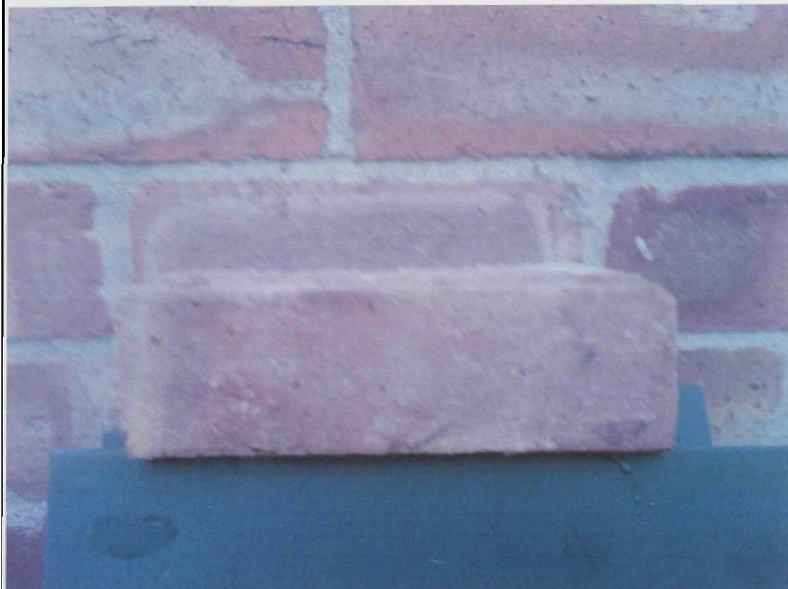
LONDON COMMON BRICKS ARE BEING USED TO MATCH EXISTING BRICK WORK
