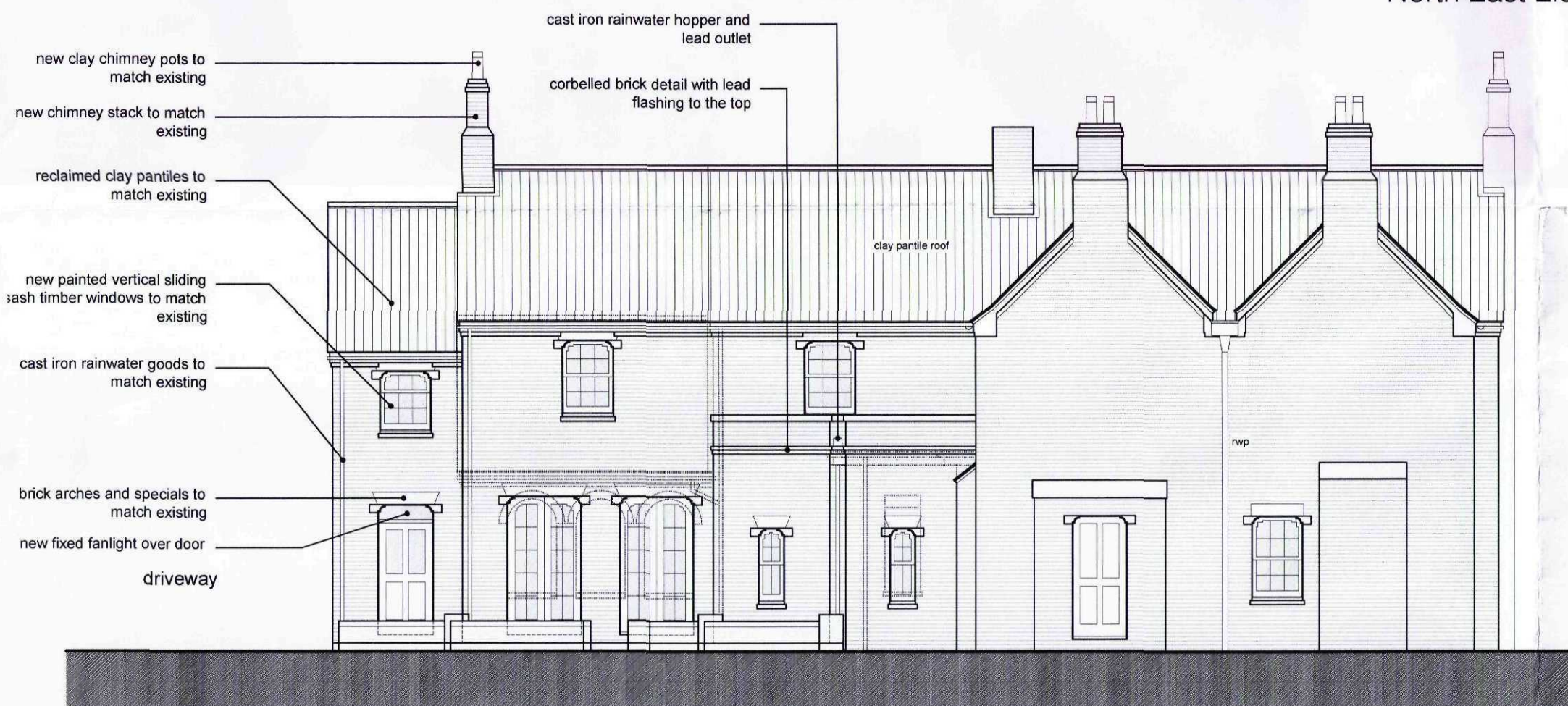
South West Elevation 1:100
