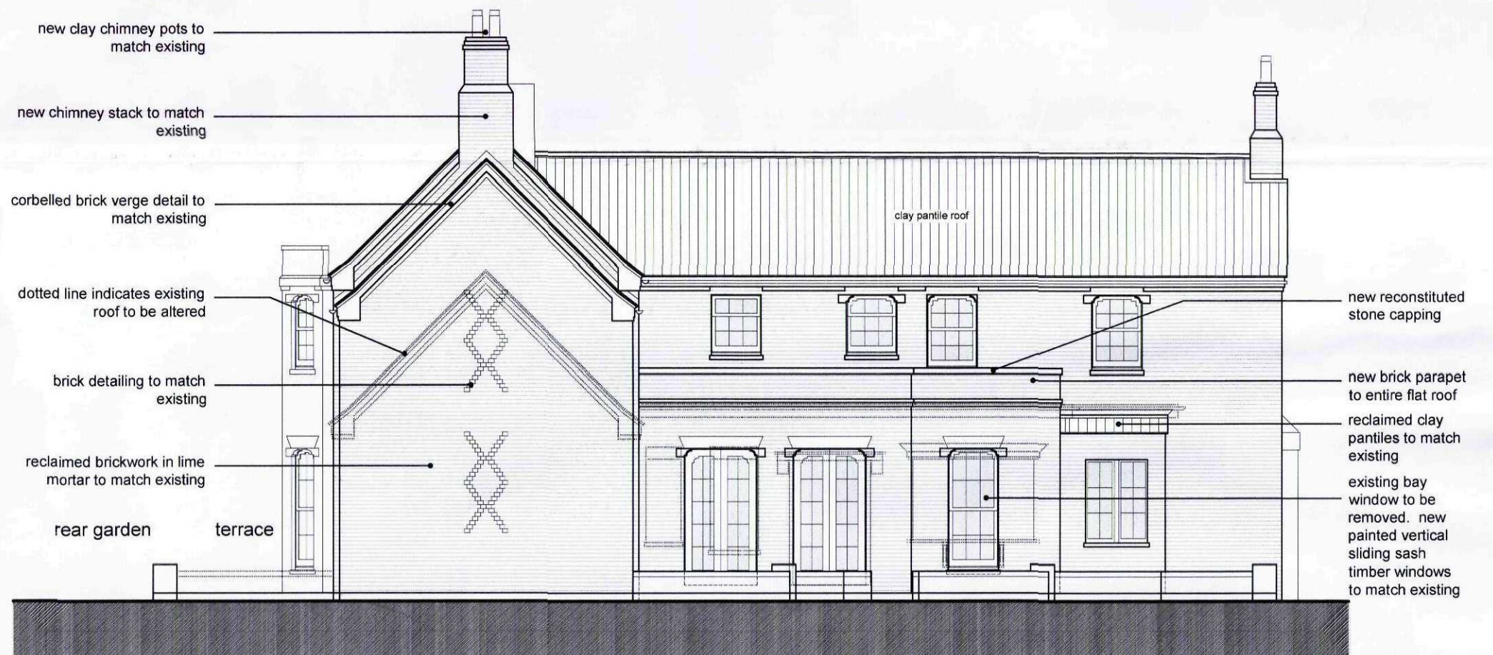
North West Elevation 1:100
