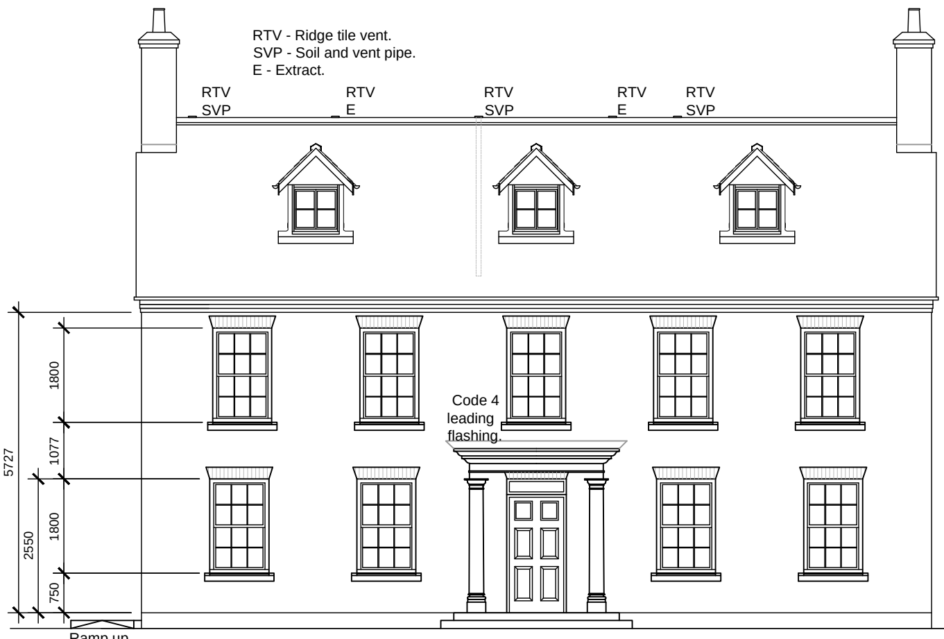
Front (south-east) Elevation
