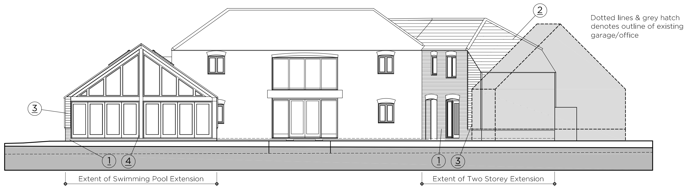
West Elevation (Front)
