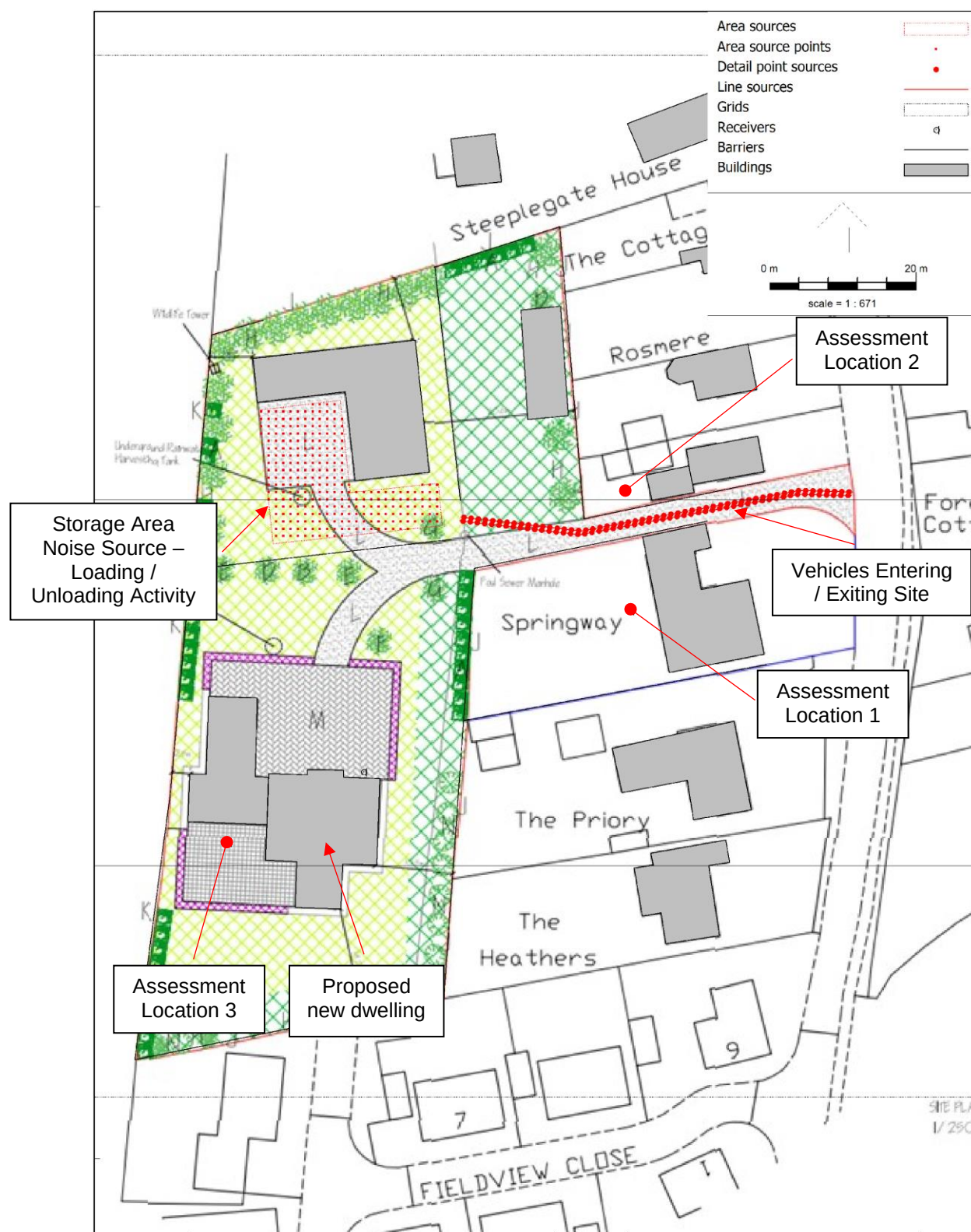
Drawing 6.1 – Computer Noise Model Showing Location Of Noise Sources and Assessment Locations
