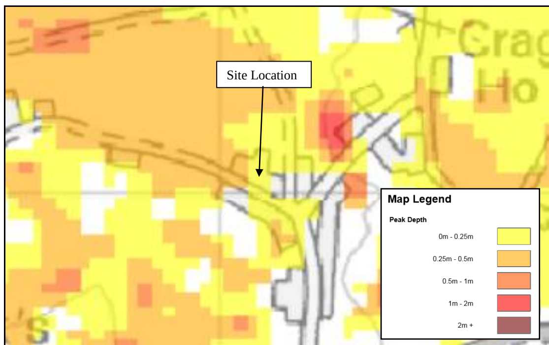
Figure 3 – SFRA 2115 Residual Peak Depth Map during the 1% fluvial and 0.5% tidal Annual Probability Event
