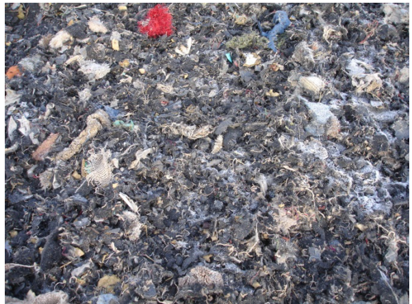
Close up view of ménage surface (recycled carpet manufactured specifically for equestrian use)
