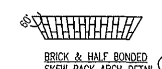
BRICK & HALF BONDED SKIN BACK ARCH DETAIL
